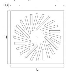
Swirl diffuser suitable for installation in rooms with a height between 2.6 and i 4.1 m, both in heating and cooling mode.
